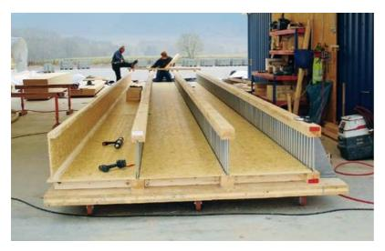
Base planking was assembled from above, avoiding the need to turn the construction elements
